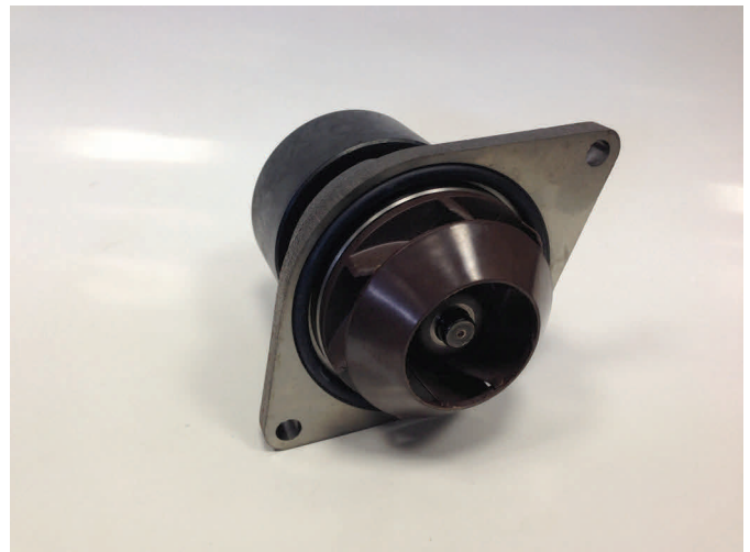
7 VANE IMPELLER Increased Coolant Flow at Low RPM HNBR Kaco Seal Seal Temp Window - 40c to + 165c
